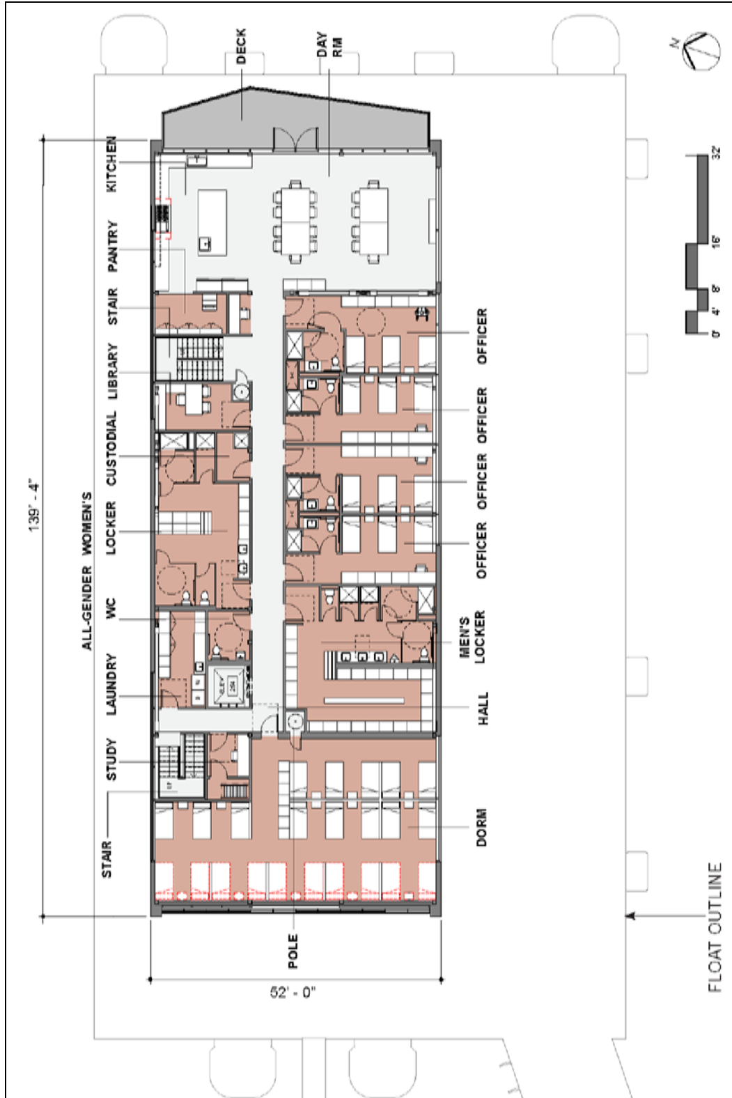
Figure 7. Fire Boat Facility Level 2
